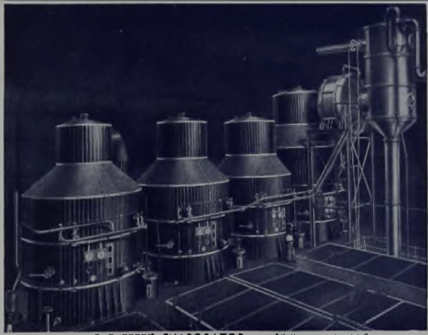
QUADRUPLE EFFET EVAPORATOR 32,000 sq. ft. H.S.
