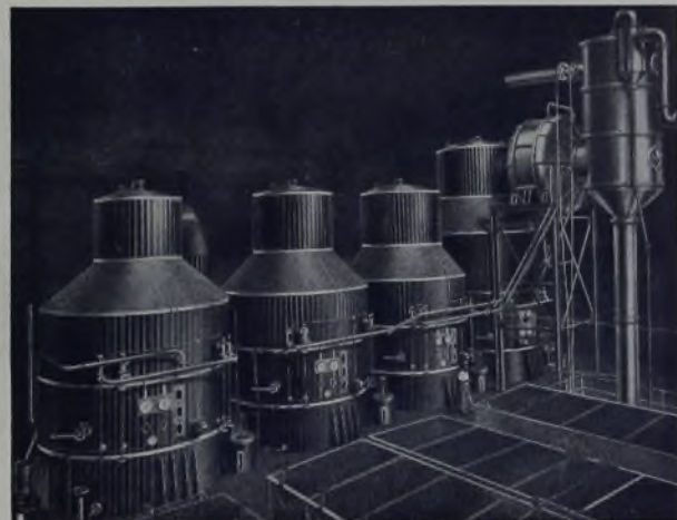
QUADRUPLE EFFET EVAPORATOR 32,000 sq. ft. G.H.S.
