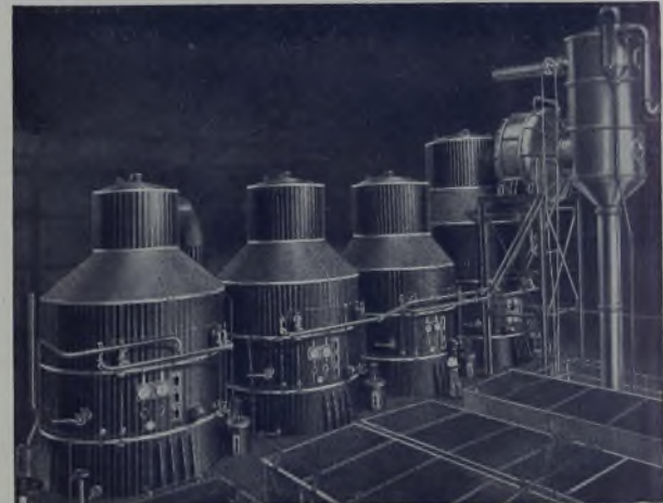
QUADRUPLE EFFLUENT EVAPORATOR 32,000 sq. ft. H.S.
